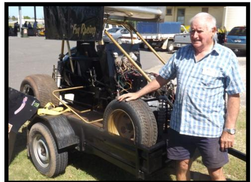
His machine has a 1,000 cc Suzuki motor bike engine which he used to race in the 1litre sprint car category. Kev still displays the old machine at speedway meets and he keeps up with the 2 litre vehicles which cost twice as much.
